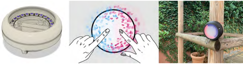
Figure P4.1: Left image shows components of El Corazón. Middle image shows the moment ending the liminal phase: recorded heartbeats are transferred into light. Right image shows El Corazón in real setting during one evaluation session.
